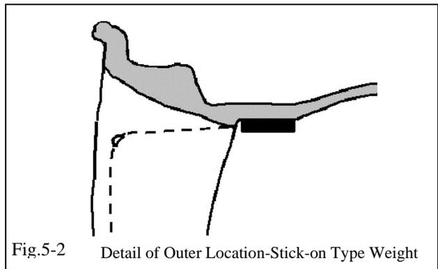
Fig.5-2 Detail of Outer Location-Stick-on Type Weight
